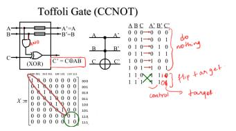
Target flipped if both control bits are set to 1. Which gate is this?
