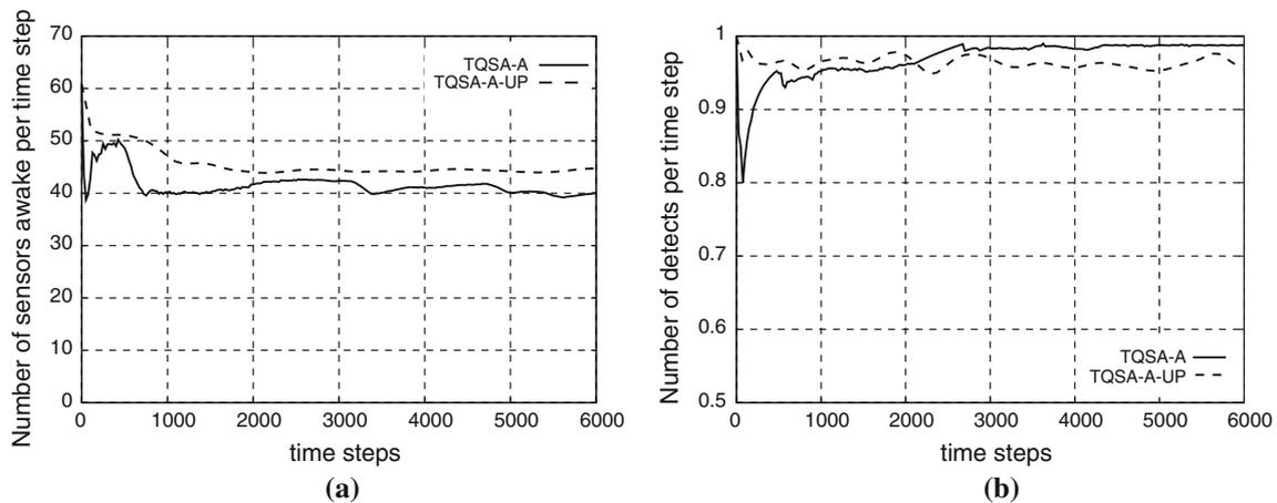
**Fig. 7** Tradeoff characteristics for TQSA-A algorithm with known and unknown  $P$ . **a** Number of sensors awake per time step. **b** Number of detects per time step
