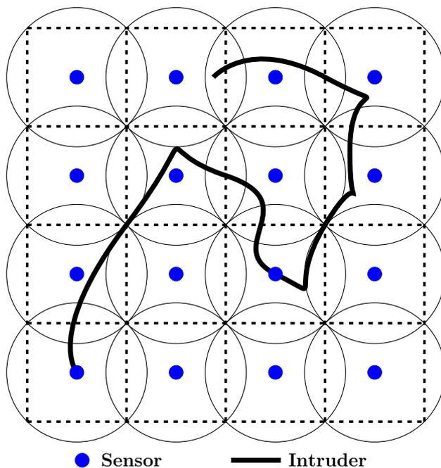
**Fig. 1** Field of sensors and the movement of intruder considered
