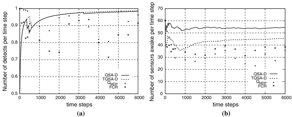
**Fig. 5** Tradeoff characteristics in the discounted setting. **a** Number of detects per time step. **b** Number of sensors awake per time step
