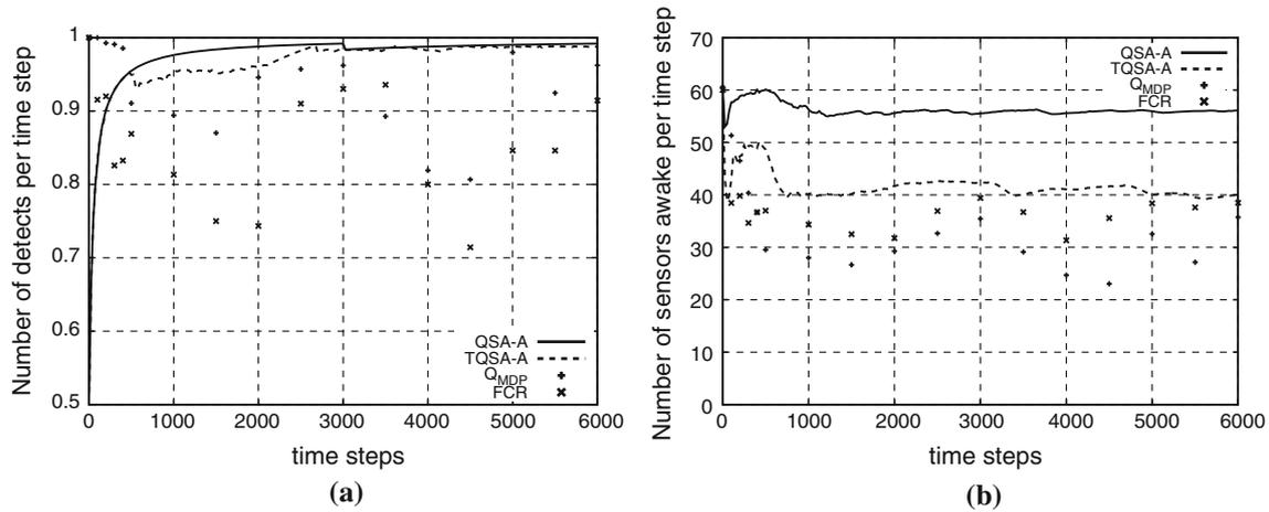
**Fig. 4** Tradeoff characteristics—known mobility model ( $P$ ) case. **a** Number of detects per time step. **b** Number of sensors awake per time step
