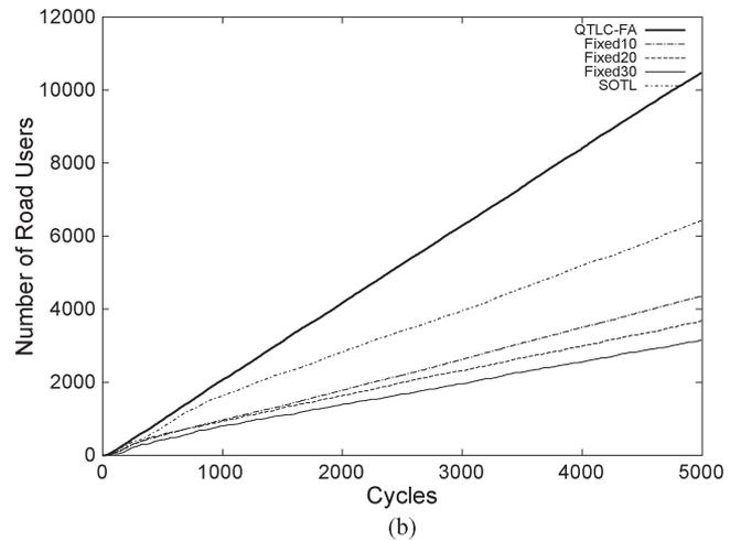
Fig. 2. Performance comparison of the TLC algorithms for the two-junction corridor case. (a) AJWT. (b) TAR.
